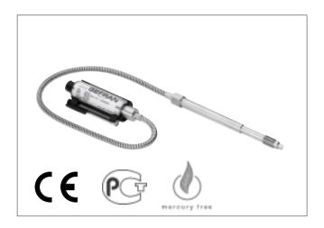
The KN Series are for use in high temperature applications where the process temperatures may reach 538°C (1000°F) such as high temperature engineered polymers. The K Series utilizes standard melt pressure principles and construction, but uses a near incompressible NAK (Sodium Potassium) for pressure transmission. The K Series strain sensing technology is bonded foil strain gage.
